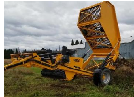
Emptying the rock bucket1
